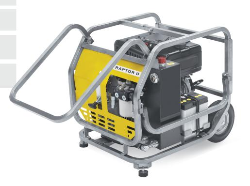
**RAPTOR D** is an hydraulic power pack with 10,5 Hp Diesel engine with electric and recoil start, it can supply an hydraulic flow from 20 to 30 L/min @ 130 Bar adjustable by the manual accelerator. **RAPTOR D** is an ideal power pack for long lasting application thanks the high efficiency oil cooling system and Diesel engine.
